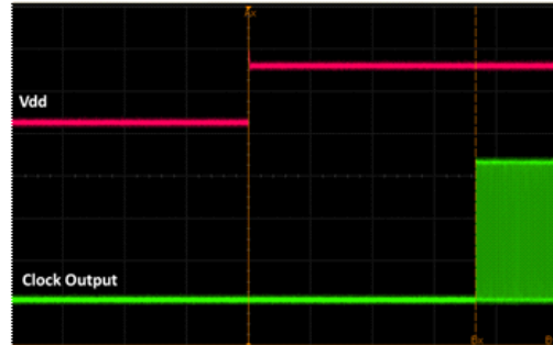
Figure 17. Startup Waveform vs. Vdd
